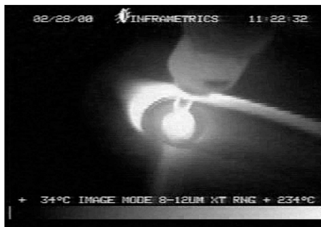
Infrared image of a duplex stainless-steel weld obtained in real time during a synchrotron experiment.
