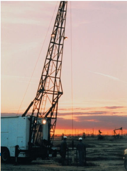
At the Lost Hills oil field, the receiver truck has lowered the underground sensor deep into the receiver well to detect the electromagnetic currents given off by the transmitter tool. The truck contains equipment for signal reception and data processing. Lawrence Livermore technicians Duane Smith (left) and Pat Lewis stand by the truck.
