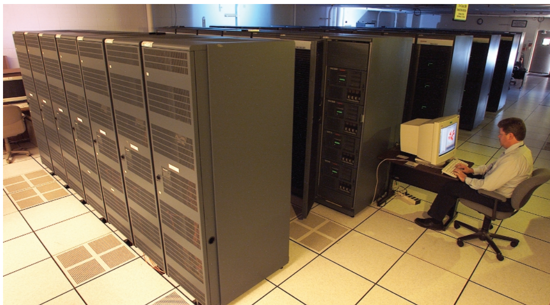
The TeraCluster2000 (TC2K) Compaq supercomputer, operating at 0.7 teraops (trillion operations per second), has 512 central processing units arranged in 128 nodes, 256 gigabytes of memory, and 10 terabytes of disk space.
