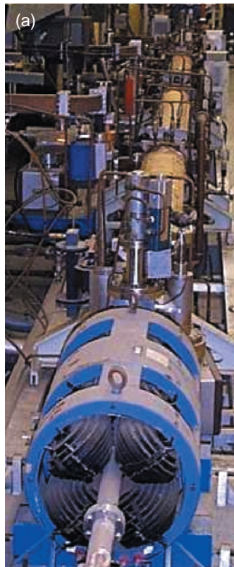
(a) The 100-megaelectronvolt linear accelerator and (b) the Falcon ultrashort-pulse laser are being integrated to produce a short-pulse x-ray source. Livermore scientists will use the x rays to probe the dynamics of materials under shock conditions.
