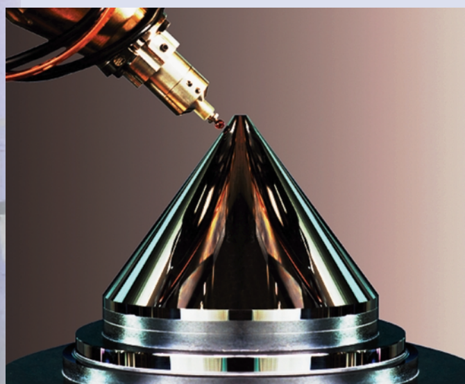
An example of the aspherical mirrors that the Large Optics Diamond Turning Machine first produced.
