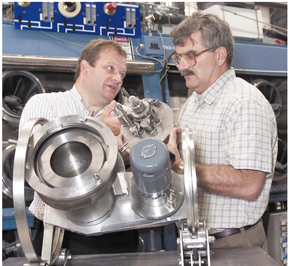
Livermore's Mark Bronson (left) and Les Jardine examine the Russian-designed and built plutonium oxide saltwasher that is being tested for use in the U.S. plutonium disposition program.
