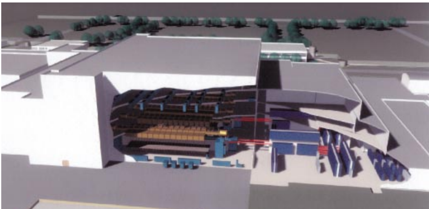
An engineering drawing of a commercial uranium enrichment plant using LIS technology. The cutaway shows banks of separators on the left, lasers on the right, and beam tubes (red) connecting the two systems.
