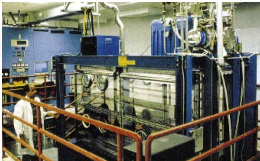
A medical laser isotope enrichment facility was built for demonstrating cost-effective separation of isotopes of interest to the medical research and medical treatment communities. The facility's separator is shown above. The dye and solid-state lasers are housed in an adjoining room.
