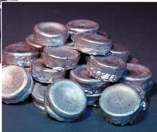
Enriched uranium produced at the Livermore pilot plant was collected as nuggets the size and thickness of several quarters. The nuggets were packed in 55-gallon drums for shipment to commercial fuel fabricators.
