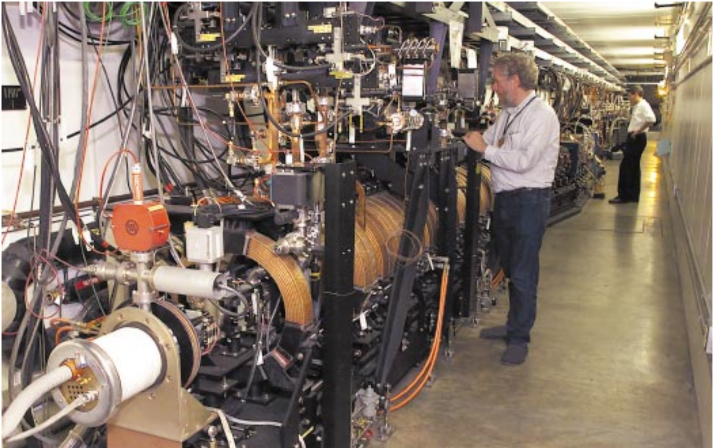
The Next Linear Collider Test Accelerator consists of a modulator to convert ac line power into dc pulses and klystrons that are driven by the dc pulses to produce radiofrequency power. The test accelerator also includes pulse compressors that reformat the radiofrequency output into 300-megawatt, 300-nanosecond-long pulses and accelerator structures that then use those pulses to establish the electromagnetic wave on which electrons surf.
