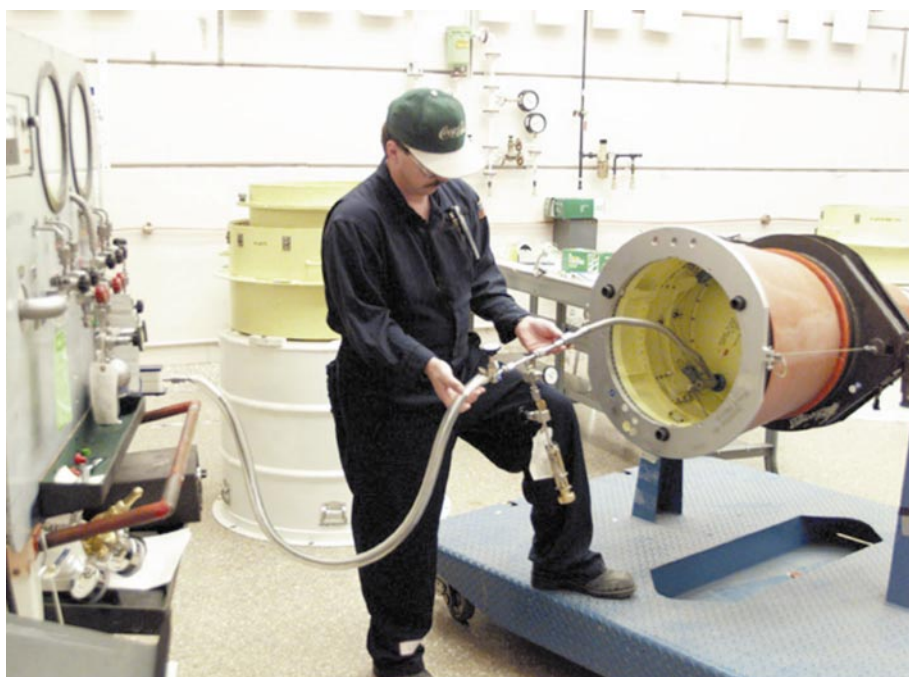
Figure 3. A technician uses an early prototype of the solid-phase microextractor (the device between his hands) to take samples of gases produced by organic materials in a weapon's headspace. Analysis of the samples provides indications of material aging.
