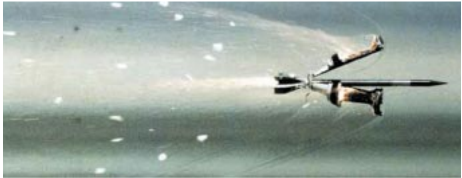
Figure 3. A sabot pushing the weapon projectile toward its target.
