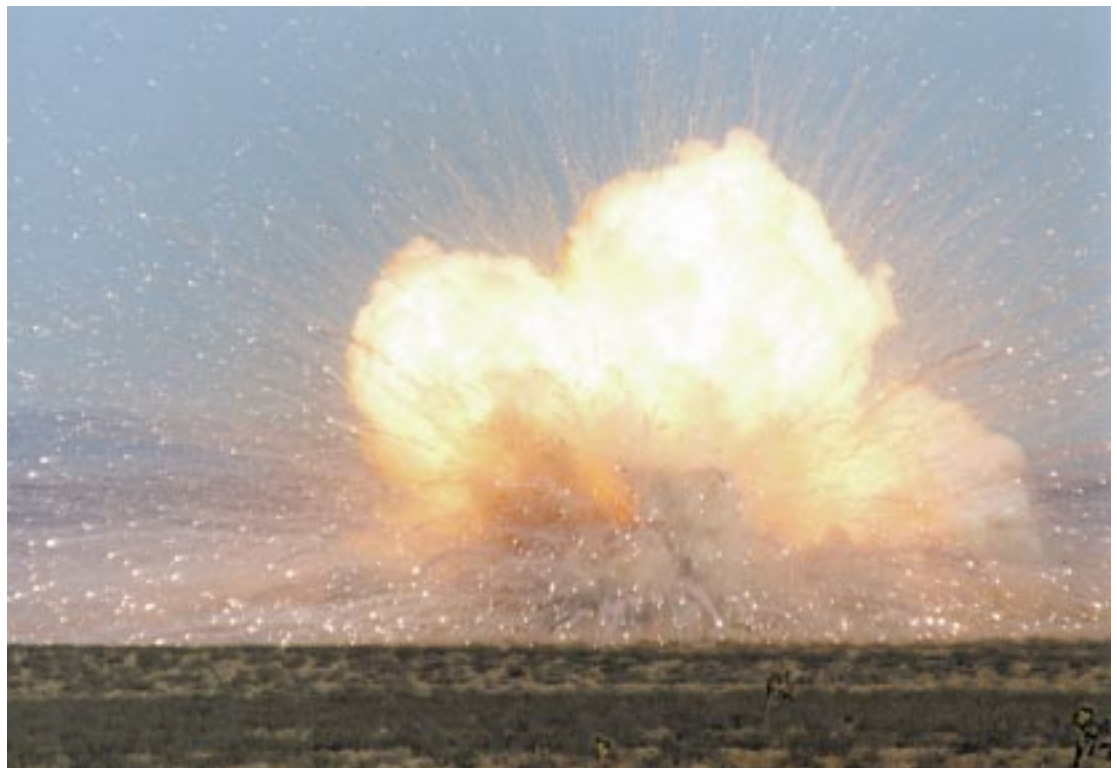
Figure 5. Data for describing the initiation and burning of explosive material are obtained through large-scale tests performed at Edwards Air Force Base, where propellants were shocked at 30,000 to 40,000 times atmospheric pressure, which caused them to explode. (Photograph courtesy of Dr. Claude Merrill, Phillips Laboratory, Edwards Air Force Base.)
