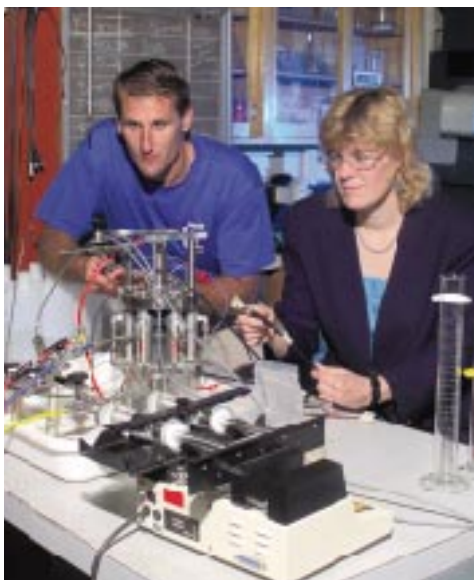
Figure 5. Pat Berge works with team member Eric Carlberg in studying conductivity and wave velocity in a range of unconsolidated sand-clay mixtures. Her team’s research seeks to discover relationships between geophysical properties and hydrogeology in the vadose zone. This basic science research is preparatory to developing a new joint inversion algorithm that environmental managers will use to directly estimate porosity and saturation in the vadose zone as part of site characterization and remediation monitoring.
