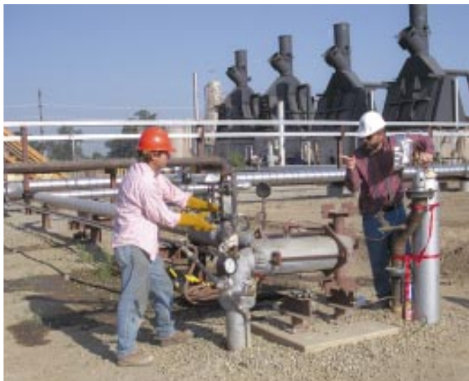
Figure 5. Livermore physicist Bryant Hudson (right), who has developed several methods for monitoring groundwater with noble-gas tracers, adjusts the gas flow with mechanical technician Allen Elsholz. Boilers are in the background.
