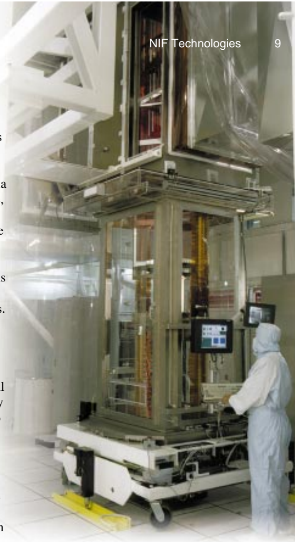
Figure 6. A technician, using a specially designed, ultraclean maintenance and assembly cart, inserts a cassette of four slabs into a frame assembly unit in the Amplab.
