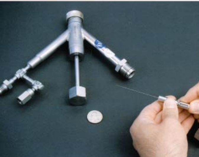
Figure 1. The relative size of the vacuum-tight microextractor assembly (left) and the coated microextraction fiber (right) compared to a quarter. The fiber is less than 400 micrometers in diameter.
