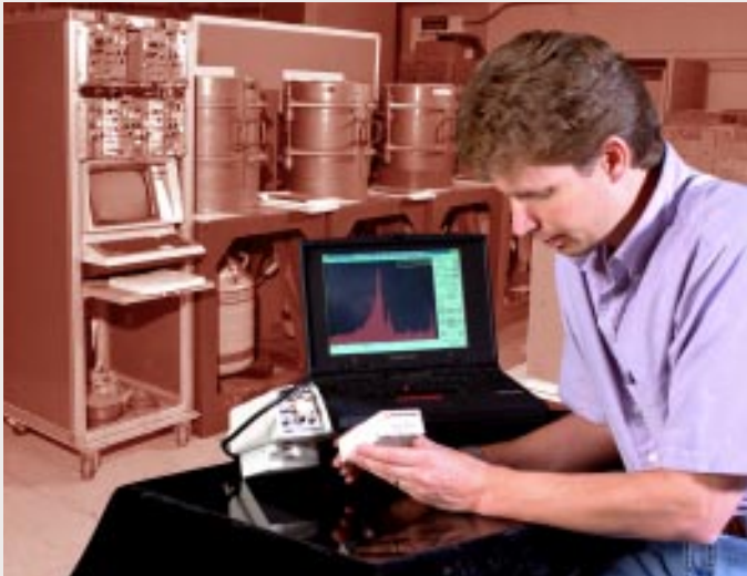
Figure 2. The portable radiation detector being demonstrated by its inventor Anthony Lavietes can identify the precise isotopic signature of nuclear materials such as plutonium and uranium by detecting gamma radiation. It improves upon the large germanium-based detectors shown in the background and has a variety of applications, among them assistance with defense against terrorism using weapons of mass destruction.
