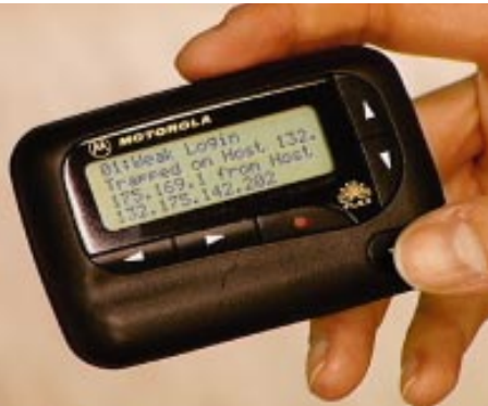
Figure 3. Currently under development by the Computer Security Technology Center, Automated Information System (AIS) Alarms allows (a and b) recognition of and (b and c) response to security incidents almost as they are happening.
