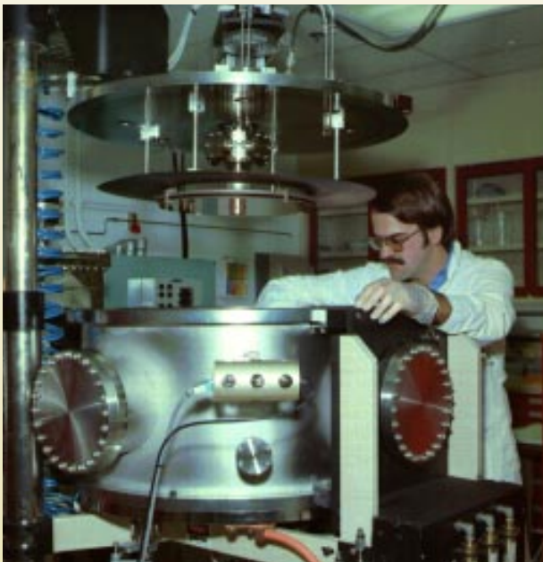
Dan Noecker of Livermore's vapor-phase deposition laboratory adjusts atom-by-atom fabrication of a new class of materials for high-strength and high-temperature applications.
