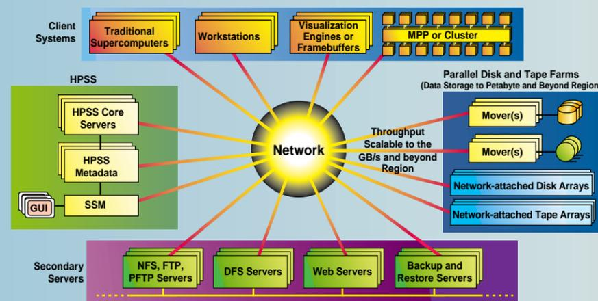
The High-Performance Storage System connects the storage units directly to a high-speed network. This network-centered architecture allows the data to flow directly between client systems and storage units, bypassing the storage server. Throughput may exceed the rate of a billion bytes per second.
