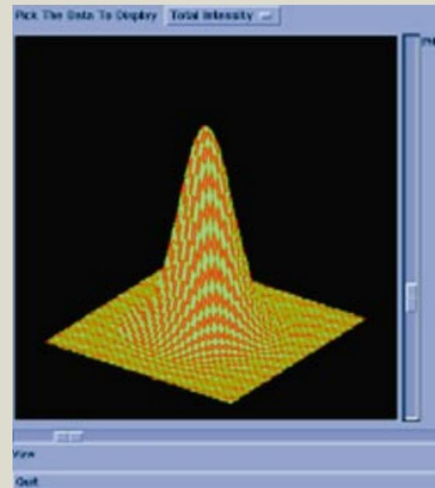
The designs of fiber-optic communication systems demand crucial calculations such as this one. Here, MELD displays the intensity profile of light propagated from a laser diode through a ball lens.
