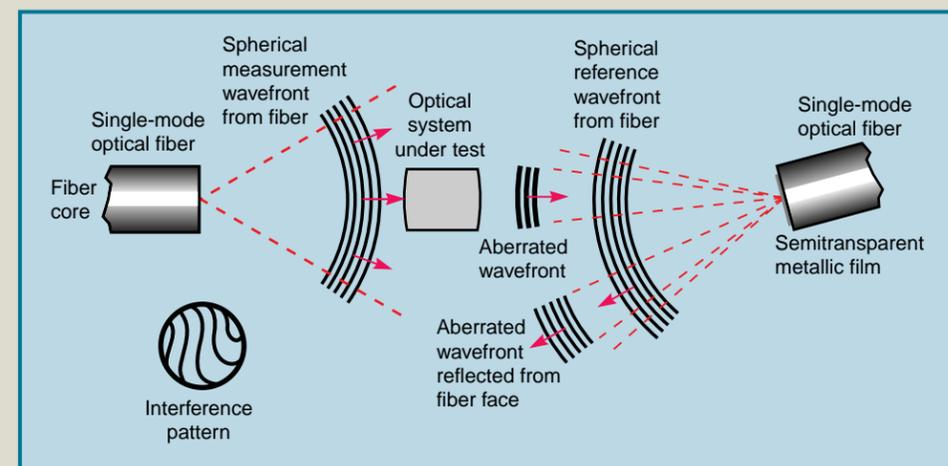
This schematic (not to scale) shows how the Absolute Interferometer operates using single-mode optical fibers. In this example, the interferometer is testing an imaging lens, but the setup is similar for testing imaging mirrors.
