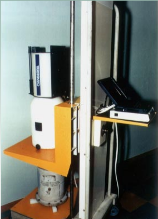
Figure 6. This prototype gamma-ray spectrometer can quickly, easily, and nondestructively determine the isotopic signatures of plutonium and enriched uranium using computer codes developed at Livermore.
