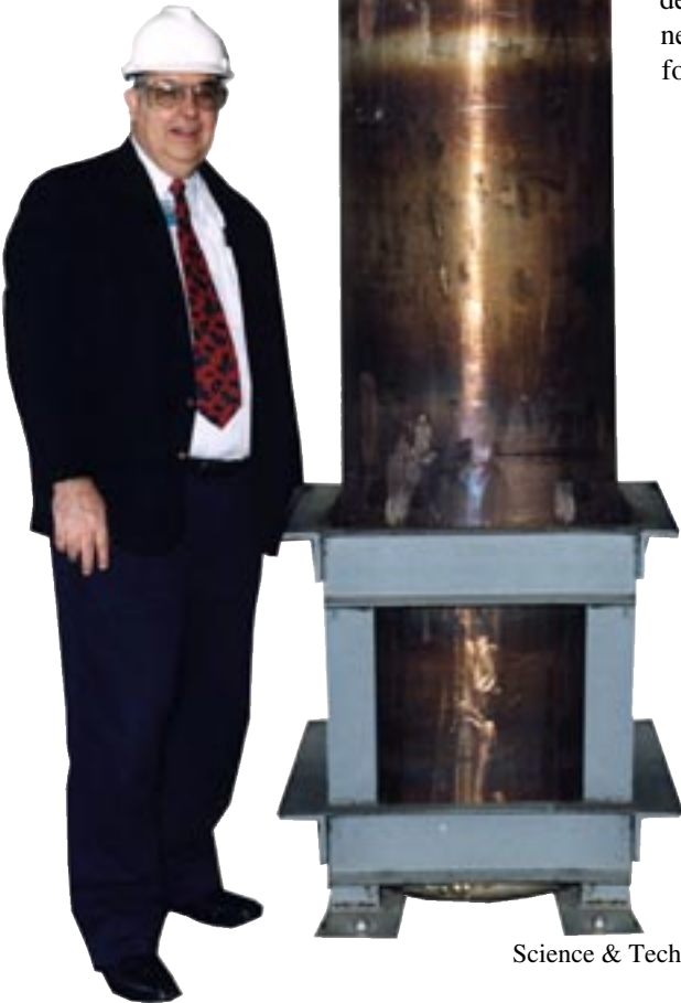
Leonard Gray, the chief scientist for Lawrence Livermore's Excess Fissile Materials Disposition Program, with a prototype stainless-steel canister, which is 3 meters (10 feet) tall and 60 centimeters (24 inches) in diameter and weighs 1,680 kilograms (about 2 tons).
