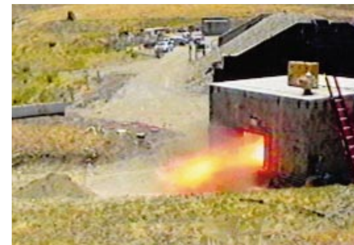
Figure 6. Detonations inside a quarter-scale model were used to determine the facility’s total structural response to future tests.
