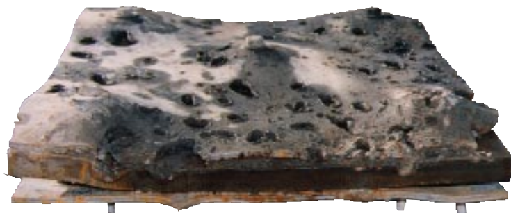
Figure 3. Shrapnel damage to a steel plate after a test to determine how much shielding is necessary for the firing chamber.
