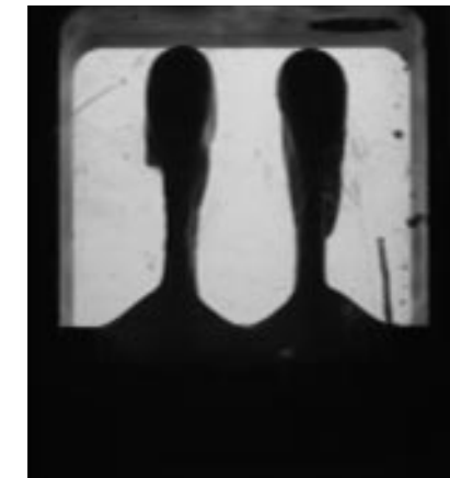
Figure 4. Yogurt perturbations after being accelerated by 30 g’s. Initial undulations at the interface were 1 millimeter; here they grew to 40 millimeters.
