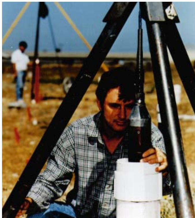
Laboratory scientist Michael Wilt sets up a field trial of crosshole electromagnetic induction technology at the University of California's Richmond Field Station. He is placing the receiver sensor in the borehole; in the background, Hung-Wen Tseng, an associate, is installing the transmitter coil.
