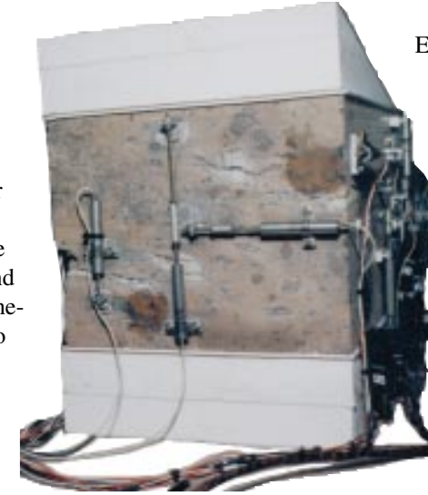
A block of Topopah Spring tuff a half-meter on a side outfitted with diagnostic instruments to study the material's responses to high temperatures and pressures.
