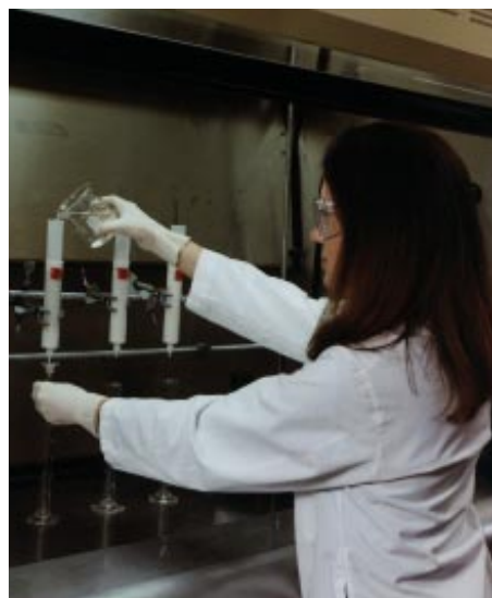
Figure 4. Researcher Cyndy Salmon uses solid-phase extraction to extract a sample by passing it through a series of small cylinders containing small amounts of organic particles.
