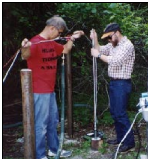
LLNL scientists recently conducted a feasibility test of the microbial filter concept at the Kennedy Space Center in Florida. This work revealed that aerobic bacteria can degrade chlorinated and fluorinated hydrocarbons under the conditions present at the site.
