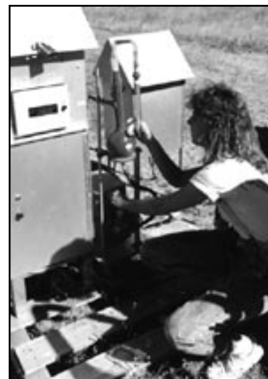
Air-monitoring stations are part of LLNL's environmental surveillance network.
