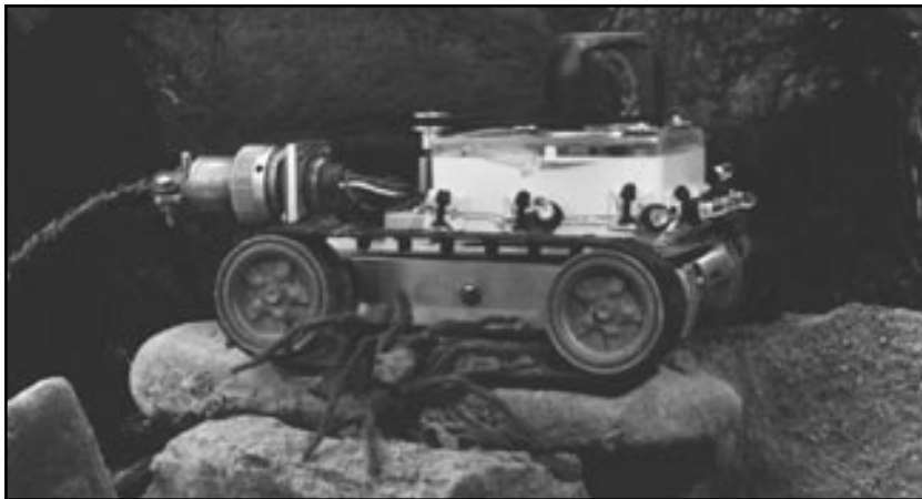
The truck-mounted miniature optic lair explorer (MOLE) is used to locate, identify, and protect endangered animals at Site 300.
