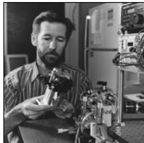
Mechanical engineer Don Masquelier works on a miniaturized flow cytometer, which uses fiber-optic data collection inside the flow stream. Compared with conventional flow cytometers, this instrument's novel signal-detection system yields a signal that is less noisy and an order of magnitude stronger.
