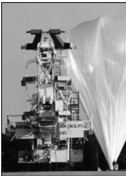
The TAISIR and GRATIS instrument package just before launch on a high-altitude balloon. TAISIR provided high-resolution images of thermal emissions on the Earth from space, while GRATIS provided images of astronomical gamma-ray sources.
