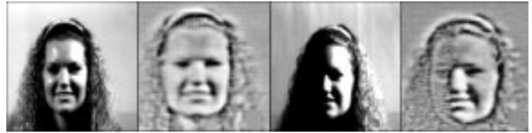
The silicon retina extracts object information from the unilluminated face area that cannot be gathered by the CCD camera. Left to right, compare the images taken in two-sided illumination by the CCD camera and silicon retina with the pair taken in one-sided illumination by the CCD camera and silicon retina.
