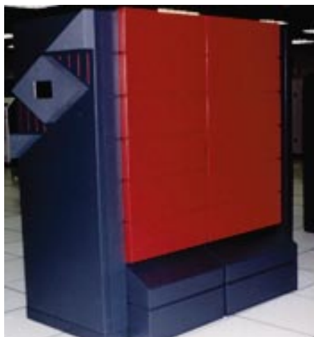
Figure 3. The CRAY T3D after its recent installation at LLNL. This massively parallel computer includes a high-performance, 88-Gbyte disk subsystem. The memory of the T3D is logically shared, but physically distributed, within a three-dimensional toroidal array of nodes. All system memory is directly accessible to all 128 processors. Each microprocessor provides 150 Mflops of peak performance. The number of processors and the disk capacity will be doubled in December for the benefit of LLNL and University of California researchers.
