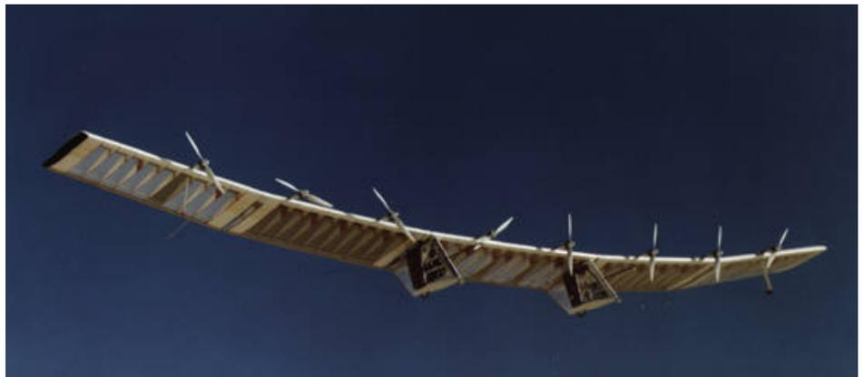
**Figure 2.** (a) Pathfinder on Rogers Dry Lake Bed before flight. The dark areas are the solar cells. Compare the slight droop of the wing with its position in (b), which shows Pathfinder in flight (altitude ~60 m). The upward curve of the wing results from lift, and this curvature of the wing puts its structural components in the condition of least load. However fragile Pathfinder might look, its flexibility and light weight allow it to withstand high wind gusts as it climbs to high altitude.
