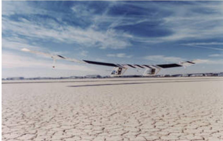
*Recent flight tests of the Pathfinder (shown above) demonstrated the potential benefits of solar-rechargeable aircraft. Since the Pathfinder is nonpolluting and very smooth flying, it offers a unique platform for high-altitude surveillance and atmospheric sensing.*
