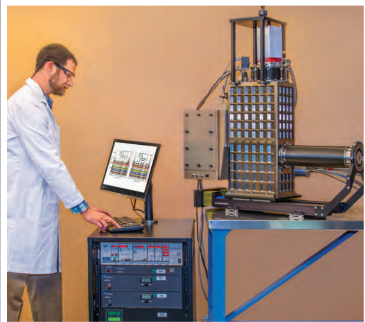
Carpenter analyzes high-resolution spectra from the STJ x-ray spectrometer (shown on the table) to characterize a material sample. The rack contains the support electronics for spectrometer operation. (Photo by Roy Kaltschmidt of Lawrence Berkeley National Laboratory.)
