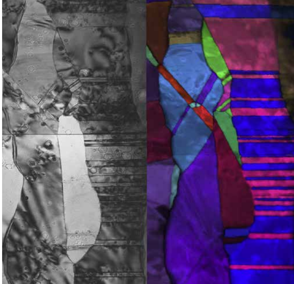
(left) A TEM image shows the topology of grain boundaries in nanocrystalline copper subjected to radiation-resistance testing. (right) Arbitrary colors used to highlight grains reveal radiation-induced voids clustering near the highly ordered, parallel-sided boundaries of grains colored magenta.
