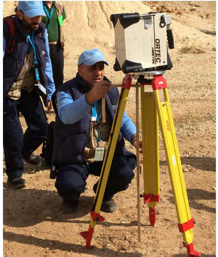
In IFE14, the ORTEC Detective, a germanium-based detector featuring Livermore's electromechanical cooling system and easy-to-use analysis interface, helped inspectors survey vast areas and identify sources of interest.
