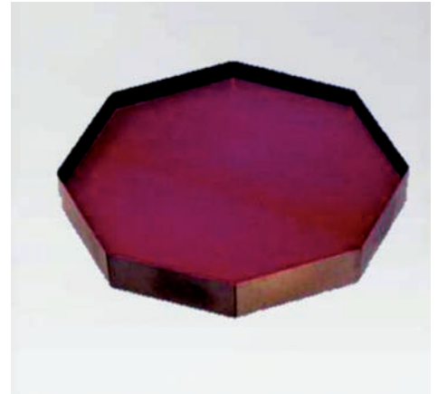
HAPLS's short-pulse laser will use (a) titanium-doped sapphire crystals as its amplification medium. (b) This polished boule measures 107 millimeters in diameter and 46 millimeters thick. (c) After the boule is sliced, it is precision cut to the desired shape, and an edge cladding is applied to suppress parasitic lasing.
