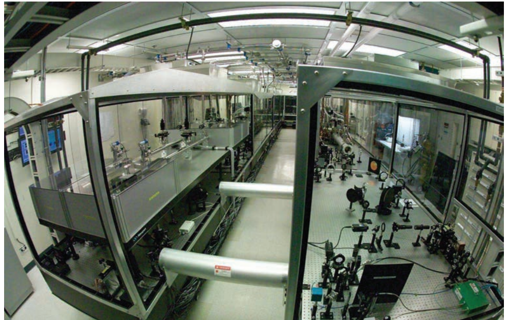
Laser diodes on the pump laser for HAPLS are key to firing 10 times a second for hours at a time. Diode technology was first demonstrated on Mercury (shown above), a high-average-power, solid-state laser system that Livermore researchers built in the late 1990s to develop and demonstrate laser fusion-energy technologies.
