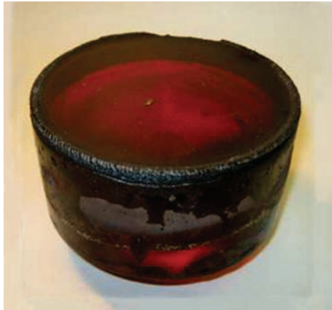
HAPLS's short-pulse laser will use (a) titanium-doped sapphire crystals as its amplification medium. (b) This polished boule measures 107 millimeters in diameter and 46 millimeters thick. (c) After the boule is sliced, it is precision cut to the desired shape, and an edge cladding is applied to suppress parasitic lasing.
