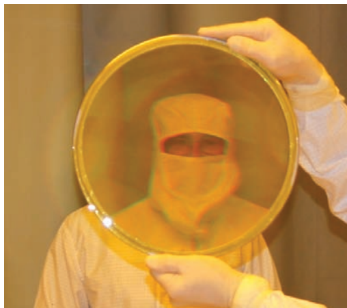
(left) Three-dimensional atomic force microscopy (AFM) is used to image the surface of a four-level glass master optic. The vertical scale (690 nanometers high) and sidewall slope is exaggerated by software and the AFM tip width, respectively. (right) With a four-level etched membrane pattern, light is diffracted in one direction, producing a single offset image of optics engineer Jerry Britten.
