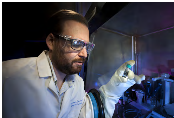
Livermore materials scientist Lars Voss holds a vial containing selenium-iodine. This semiconducting material may be useful for developing long-lasting, reliable radioisotope batteries. (Photo by Randy Wong.)
