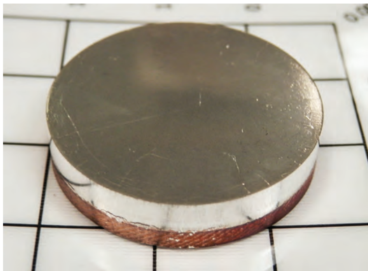
(left) The graded-density impactor (GDI) combines up to 100 metallic layers of varying densities. This particular GDI comprises copper on the bottom, a combination of copper and magnesium in the middle, and magnesium on top. (right) The GDI is pressed into a plastic case to create the complete "bullet" (about 3.8 centimeters or 1.5 inches long) that travels down the gas gun. Only the metal plate at the top of the projectile impacts the target.
