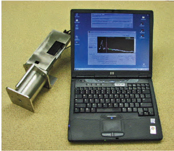
(left) The portable Livermore-developed nondestructive assay (NDA) system provides uranium enrichment measurements for the HEU Transparency Program. The low-cost, low-maintenance system is constructed of commercially available components. (right) The graph shows the spectrum of a 93-percent enriched U.S. uranium oxide standard, acquired with the portable NDA system. The count time was 300 seconds.
