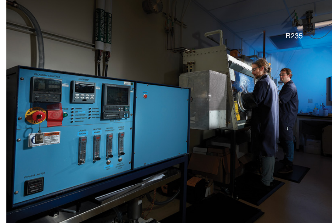
Staff scientists Logan Winston (left) and Evan Clarke (right) manipulate samples inside the Hydride–Dehydride (HDH) powder machine (above). The HDH project offers the capability to transform a raw slab of uranium alloy into rough flakes before a spheroidization produces a fine sand-like substrate for use in the development of dynamic shapes (below).
