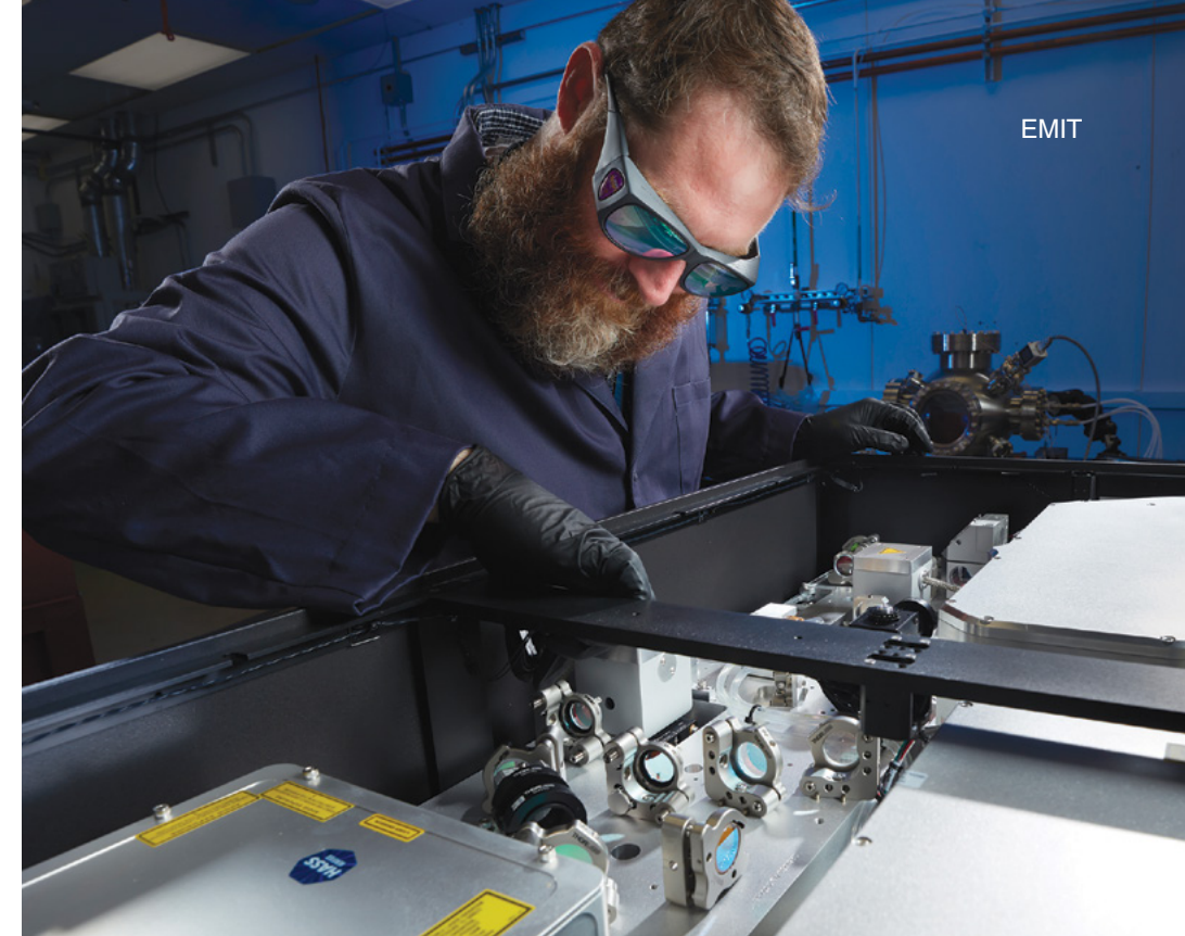
Diagnostic team lead Ben Goldberg inspects a series of mirrors under the hood of EMIT's newly acquired femtosecond laser system used to measure airflow and chemical effects.
