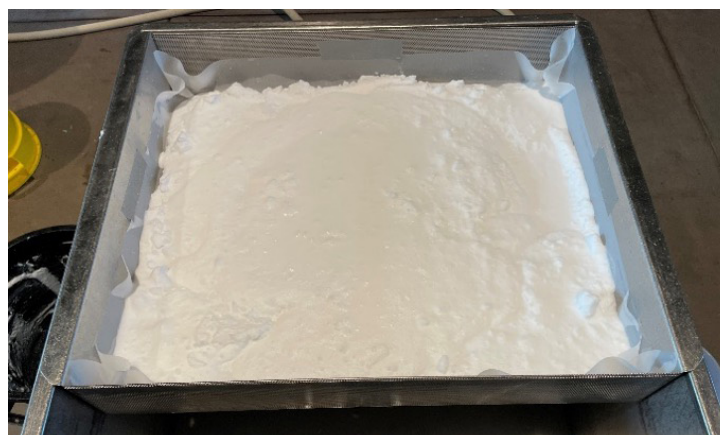
Nesquehonite, a magnesium carbonate mineral containing the sequestered CO 2 , is produced by mixing the saturated solvent with a magnesium chloride solution. Squeezing excess water from the nesquehonite results in a powdery substance safely containing the captured CO 2 .
