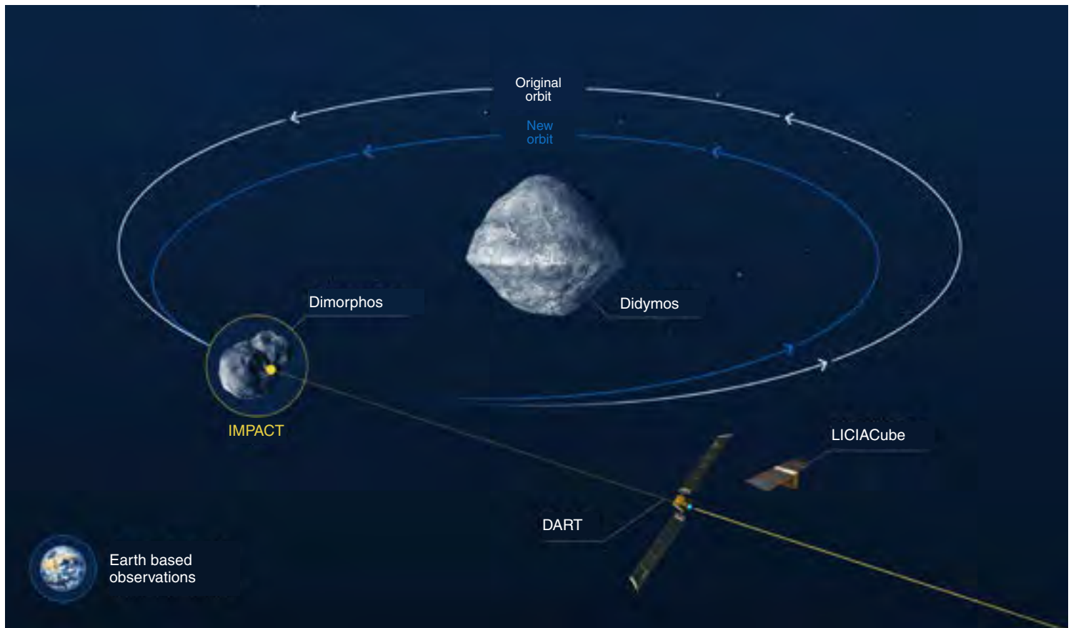
The Double Asteroid Redirection Test (DART) included observation from multiple vantage points: from Earth and, before impact, from the DART spacecraft, which also deployed the Light Italian Cubesat for Imaging Asteroids (LICIACube) to record the kinetic impact that altered Dimorphos’s orbit around Didymos. (Image courtesy of Johns Hopkins University Applied Physics Laboratory (JHUAPL).)
