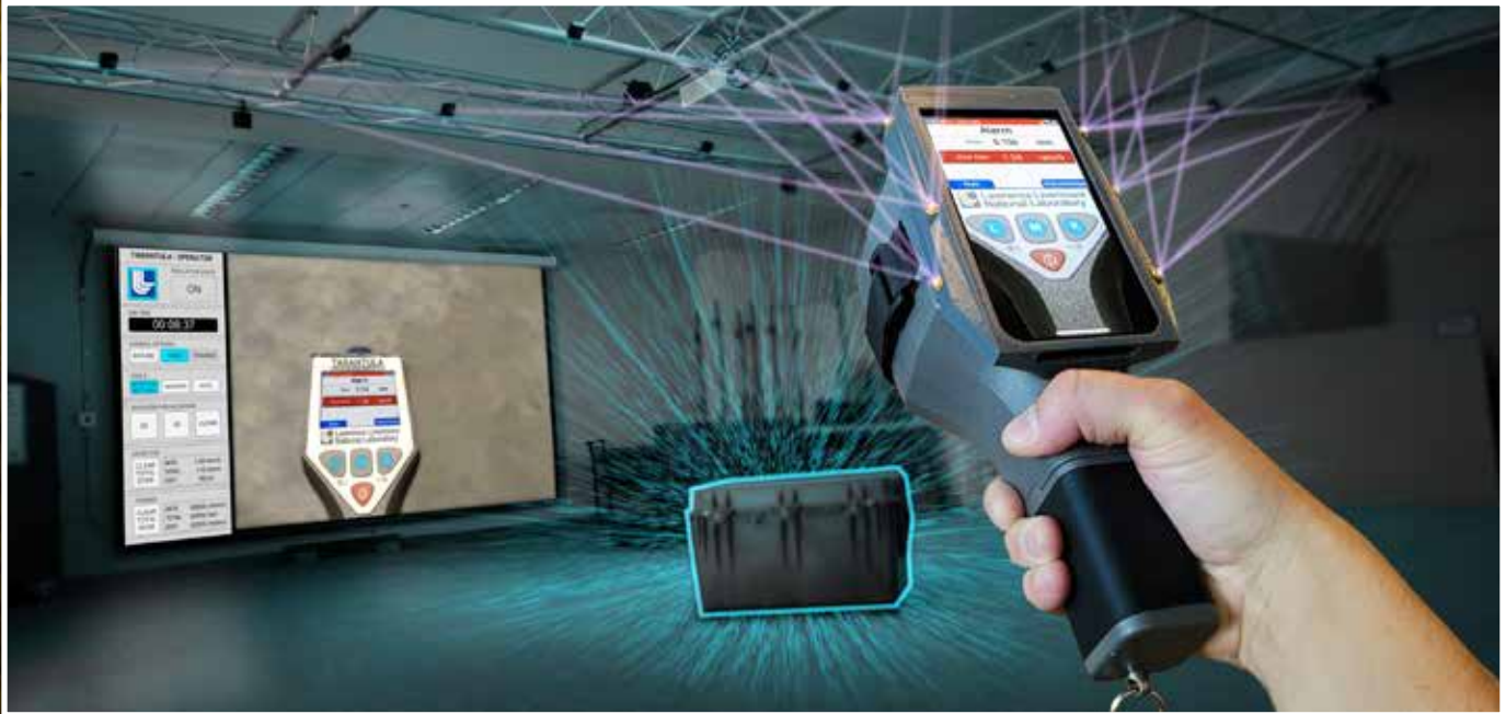
(above) This visualization shows a setup of the TARANTULA (Tactical Augmented Reality Applications for NEST (Nuclear Emergency Support Team) Training using Livermore Analytics) augmented reality (AR) platform inside a large warehouse. An array of cameras above the training area tracks a simulated detector using infrared light sources (visually represented by the path of purple lights streaming from the cameras to the markers around the edge of the detector). The simulated item of primary concern (black case) is also marked and tracked by the cameras. The screen in the background provides instructors with a real-time view of everything the trainee sees during the training exercise. (Images by Ryan Chen.)
