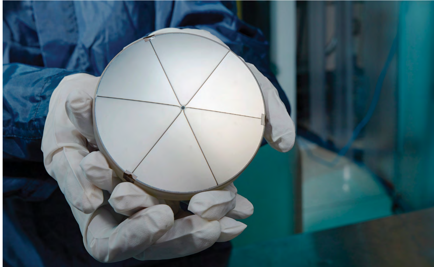
The Geostationary Operational Environmental Satellites contain the first telescopes that image at six different EUV wavelengths using a single pair of mirrors. A close-up view of a test secondary mirror (above) with six segments, coated with molybdenum-silicon and molybdenum-yttrium multilayers. Each segment is designed to reflect at a different EUV wavelength. An aperture selector in the telescope allows illumination of the specific coating segment needed to pass the desired EUV wavelength. (Photo by Garry McLeod.)
