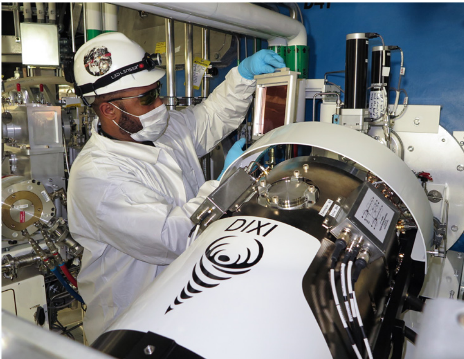
Target Area Operator Bill Board removes an image plate from the NIF Dilation X-ray Imager (DIXI), the world's fastest x-ray framing camera. It produces images of an imploding target capsule with 10 times faster temporal resolution than previous systems. DIXI is one of 120 NIF diagnostics developed for characterizing experiments in unprecedented detail. (Photo by James Pryatel.)
