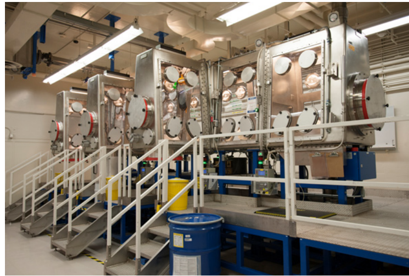
Staff in Lawrence Livermore's Radioactive Hazardous and Waste Management Program sort contaminated debris in the onsite Centralized Waste Processing Line, a large glovebox.
