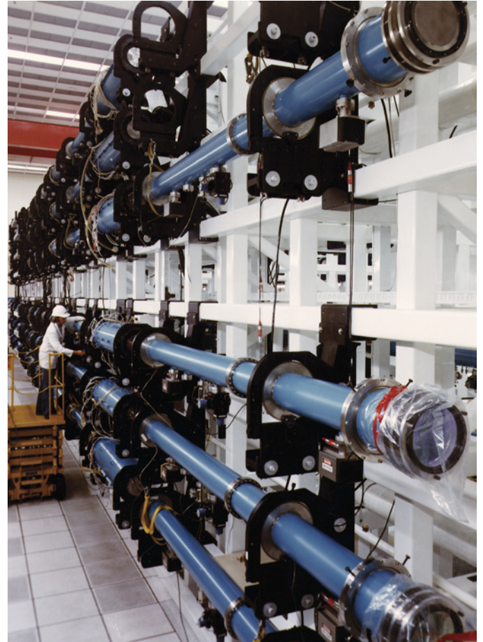
The 20-beam Shiva became the world’s most powerful laser in 1977, delivering an unprecedented 10.2 kilojoules of energy in less than a billionth of a second in its first full-power firing. Shiva’s laser bay (shown here) captures the large scale of development taking place by the late 1970s.
