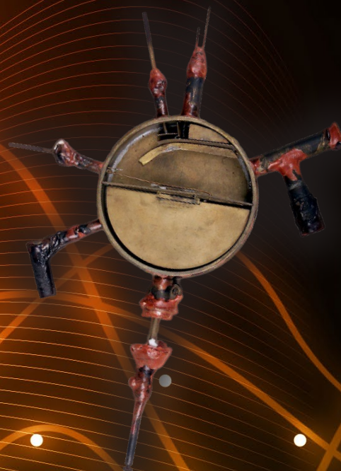
The first successful cyclotron (above) built by Ernest O. Lawrence (below) accelerated a few hydrogen ions to an energy of 80,000 electronvolts. The device earned Lawrence $500 from the National Research Council towards the construction of a machine that might be useful for nuclear physics. (Images courtesy of University of California, Lawrence Berkeley National Laboratory.)
