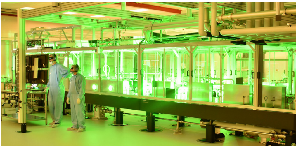
Livermore delivered the High-Repetition-Rate Advanced Petawatt Laser System (HAPLS) to the the Extreme Light Infrastructure Beamlines facility in the Czech Republic in 2017, representing the Laboratory’s expertise in high-repetition-rate petawatt laser construction.
