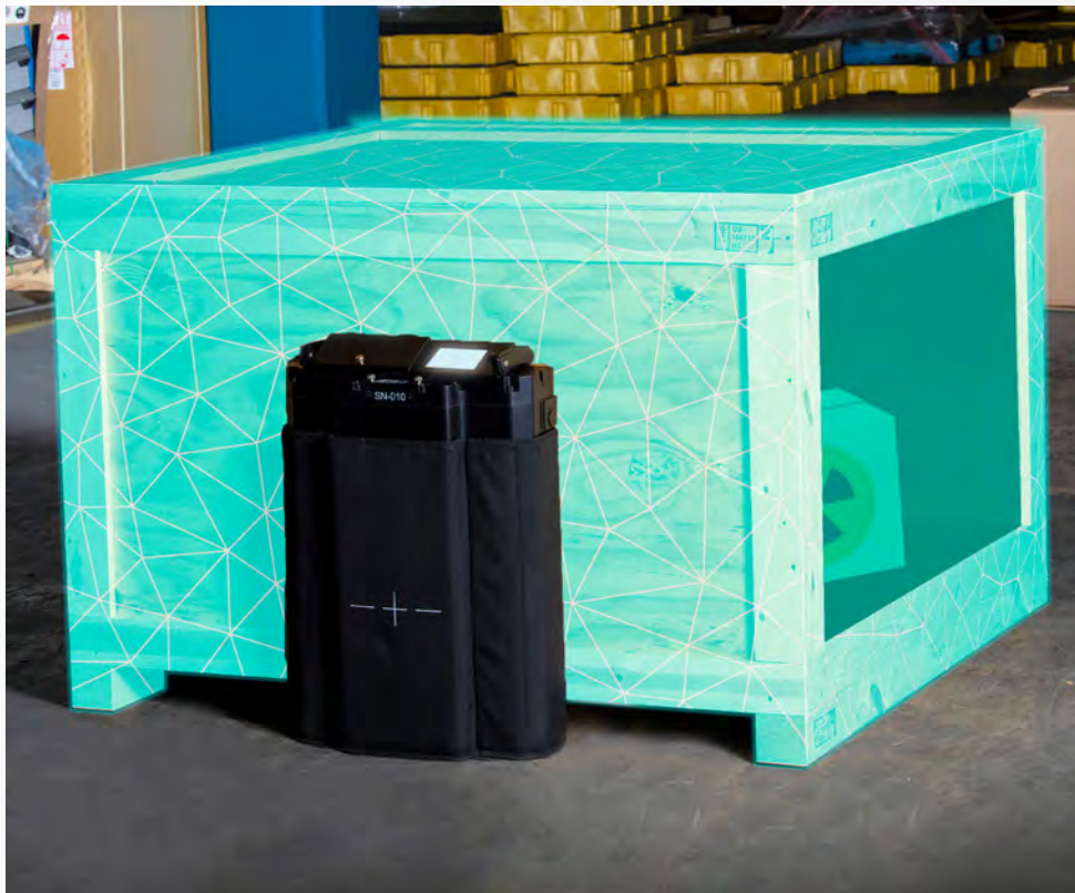
MC-15 (black box) is smaller and lighter than competitive neutron multiplicity counters and is designed to be operated in the field for real-time nuclear threat assessment.
