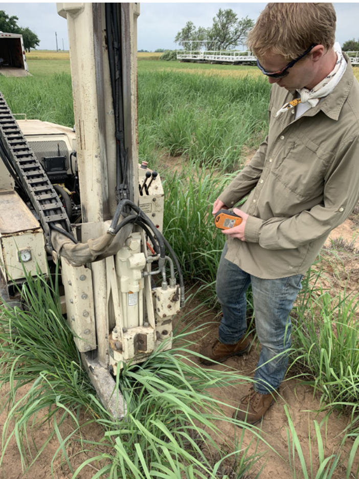
Using a Geoprobe 54LT coring device, researcher Eric Slessarev takes a 2.5-meter-long core sample to determine whether the deep rooting system of Texas switchgrass retains more soil carbon than annual crops. (Photo by Erin Nuccio.)
