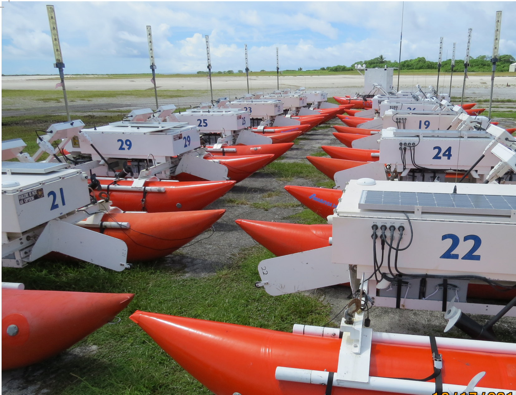
The LIDSS rafts at Kwajalein Island await transport to the area where they will gather data during the next test of a Minuteman III missile.
