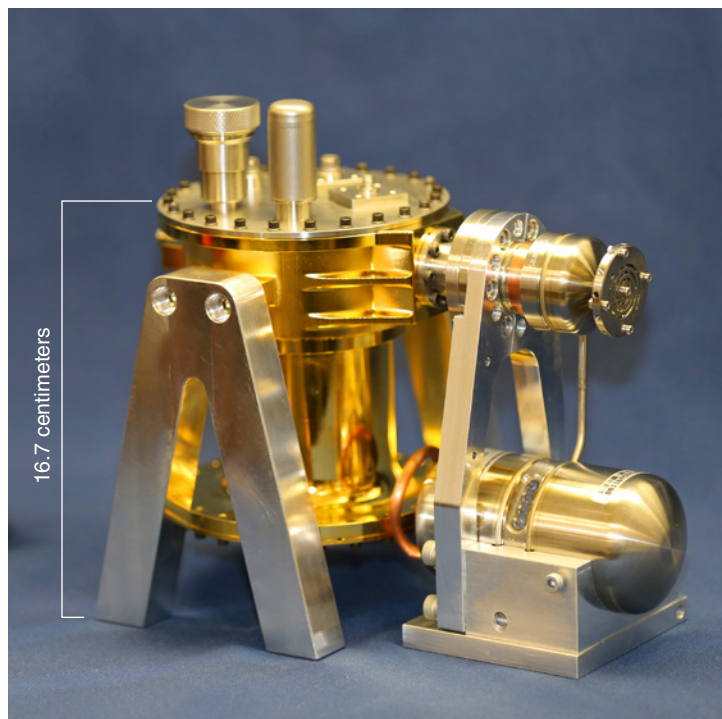
GeMini-Plus is an improved, simplified, and more rugged version of the original GeMini gamma-ray spectrometer. The enhancements make the device more versatile than its predecessor.
