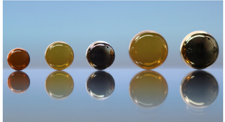
Direct-drive targets are gas-filled capsules ranging in size from 2 to 4 millimeters that contain room temperature deuterium and tritium. When heated by the laser, these capsules generate powerful 14-megaelectronvolt neutrons for survivability experiments. (Photo courtesy of General Atomics.)
