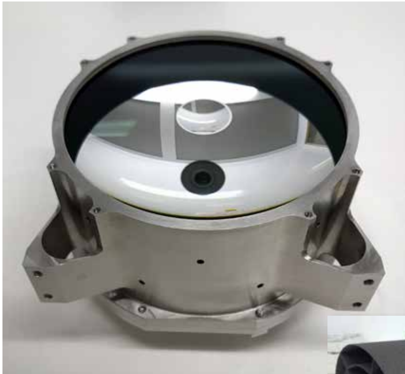
GEOstare CubeSats use monolithic telescopes, which combine the primary and secondary mirrors into a single optical element (left). The entire telescope assembly (below) also includes the baffle (black component) to reduce stray light.
