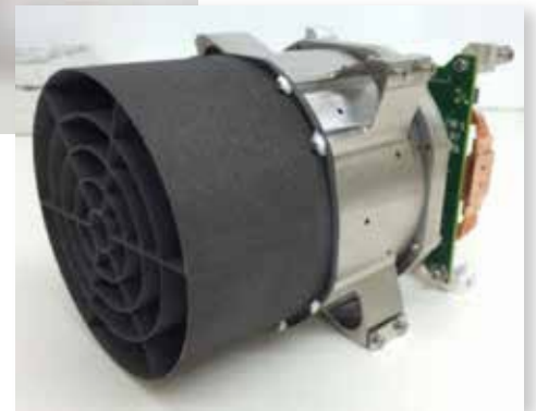
GEOstare CubeSats use monolithic telescopes, which combine the primary and secondary mirrors into a single optical element (left). The entire telescope assembly (below) also includes the baffle (black component) to reduce stray light.
