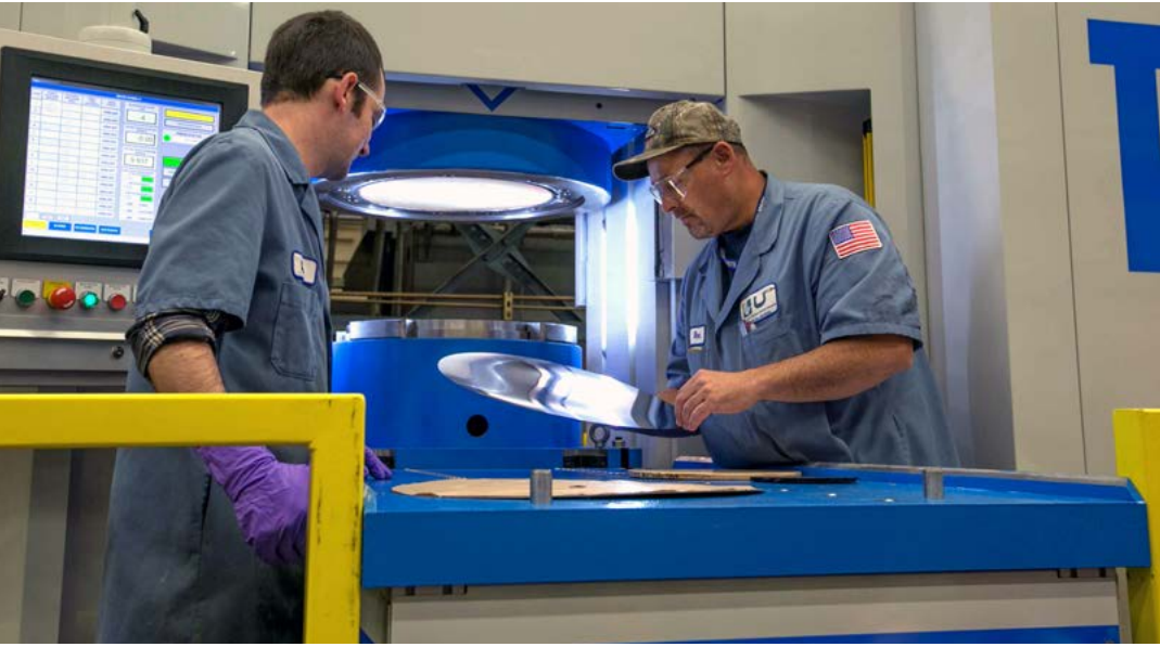
Machinists Wes Scoggins (left) and Ron Cabeceiras examine a steel sheet before pressing it into a test part with a new hydroform, the key tool for building experimental parts for the W80-4 LEP. (Photo by Julie Russell.)
