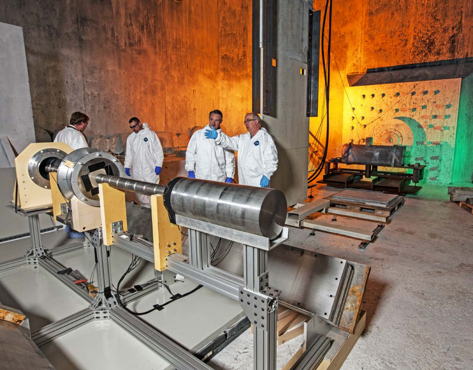
Technicians know as “ramrods” set up an experiment inside the Contained Firing Facility (CFF), the nation’s largest indoor firing chamber. Hydrodynamic experiments at CFF create extreme temperature and pressure conditions to assess the performance of nonnuclear weapon components for life-extension programs (LEPs). (Photo by George Kitrinos.)
