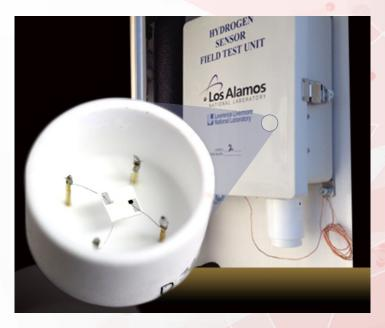
This simple and inexpensive solid-state, electrochemical hydrogen safety sensor was tested at a hydrogen fueling station run by H2 Frontier, Inc. The device meets more of the Department of Energy's performance targets than all other commercial platforms, while operating under an extreme range of ambient temperatures.
