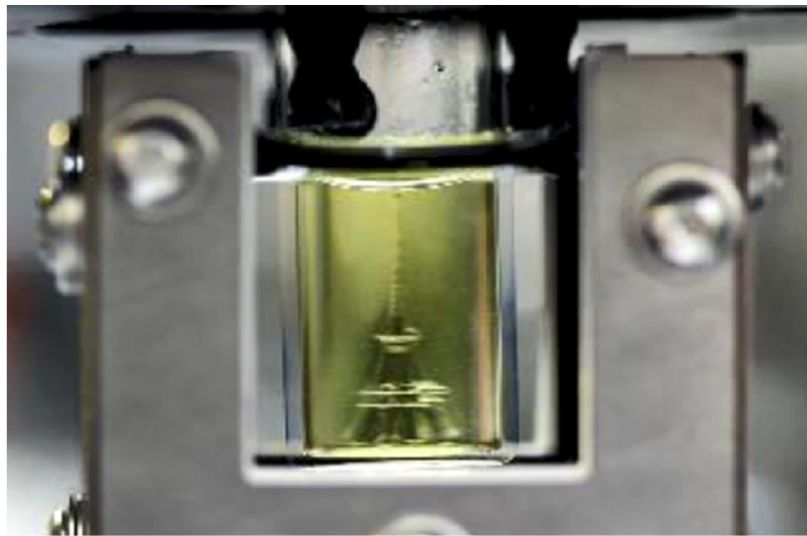
Using computed axial lithography, a 3D model of the Eiffel Tower is formed. (left) Each video frame shows the shape from a slightly different perspective. (middle) Inside a rotating chamber, the beam reacts with light-sensitive resin, which begins to harden. (right) After about 2 minutes of exposure, the resin solidifies into the 3D part.
