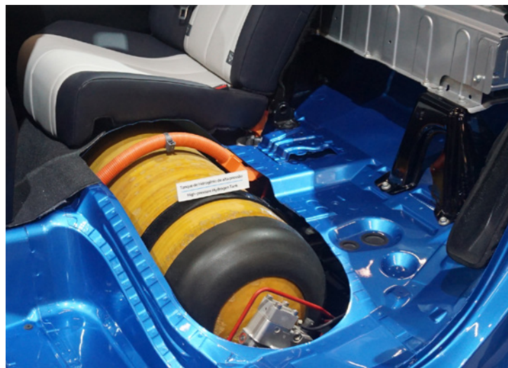
Hydrogen storage tanks for vehicles, such as the one seen here in a Toyota Mirai, are large and cylindrical. By storing hydrogen within a solid material rather than as a pure compressed gas, more hydrogen could be contained in smaller vessels that better fit automotive interiors. (Photo courtesy of Mario Roberto Durán Ortiz. Licensed with CC BY-SA 4.0.)
