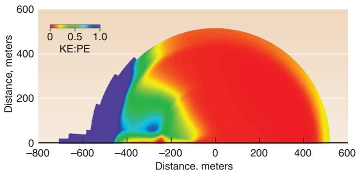
Simulation results show the effects of detonating a 1-kiloton nuclear explosive 150 meters above the surface of a 1-kilometer-diameter object. Colors indicate the ratio of kinetic energy (KE) to potential energy (PE) produced by the impact. The explosion obliterates the ejected debris (purple). In the bound areas (light blue to red), the object receives a "push," which changes its speed by a few centimeters per second.
